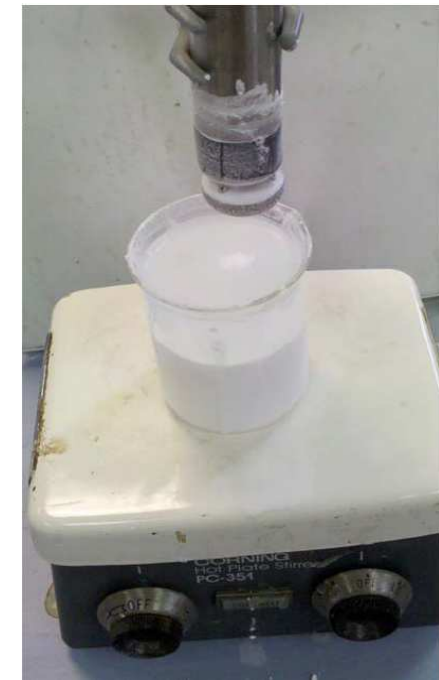
Ultrasound probe lowered into stirred slurry of inert particles
